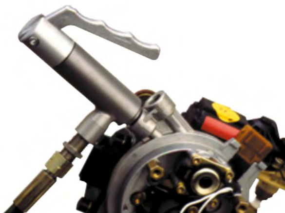
TW17H | Testing of injection pumps
